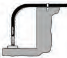
Figure 5. Hose Length Due To Pressure
